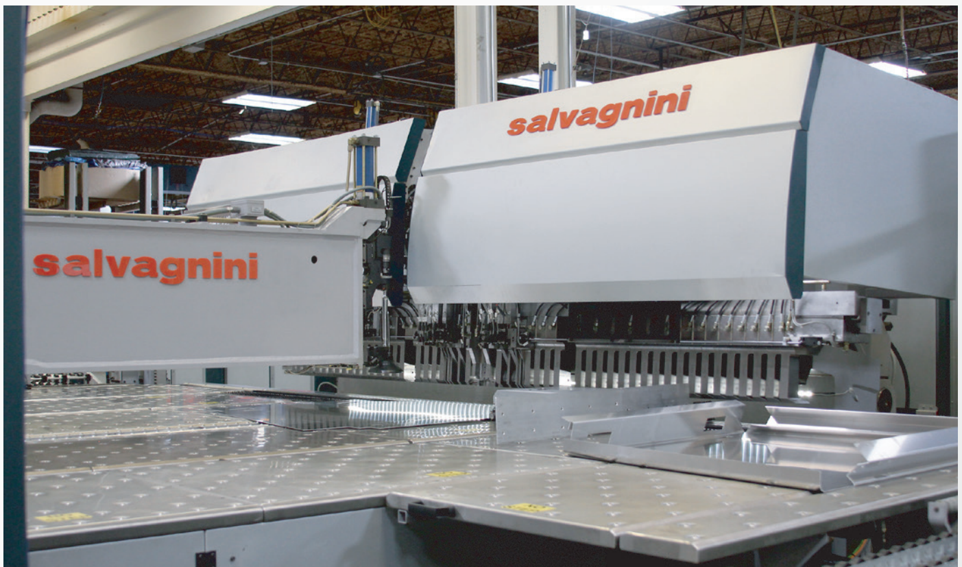
Pictured: One of our Salvagnini panel benders automatically forms a sheet into a complex part.
